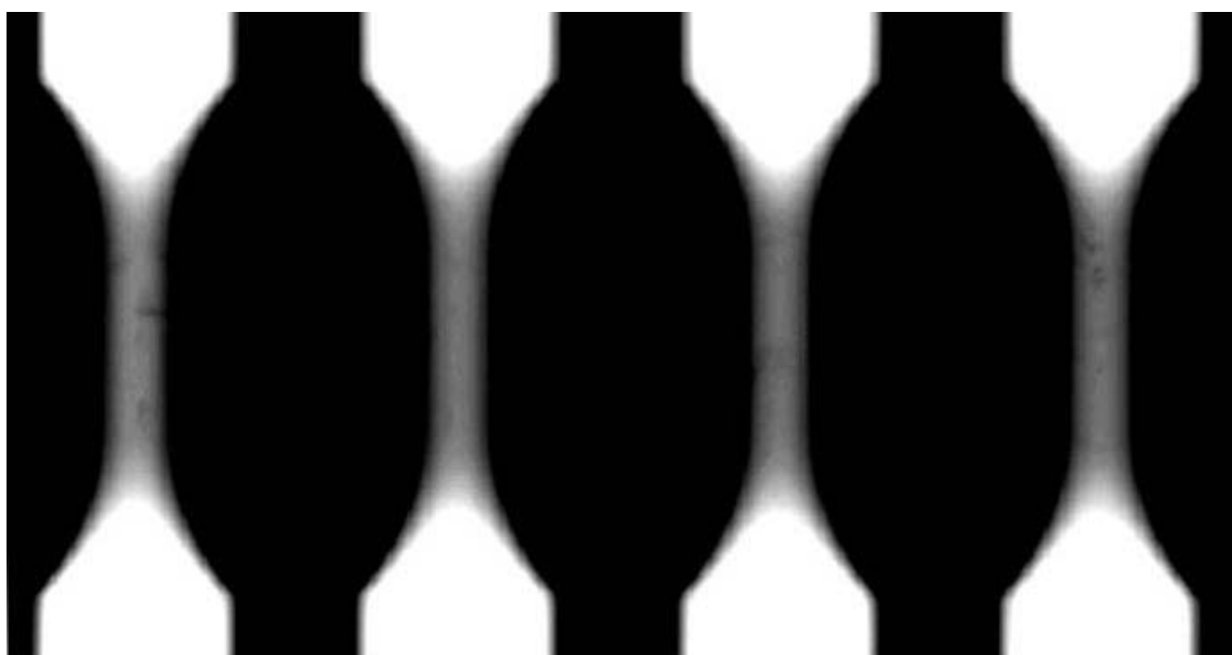
Figure 2.8 - Representative Radiographs of Straight Cylinder Specimens
