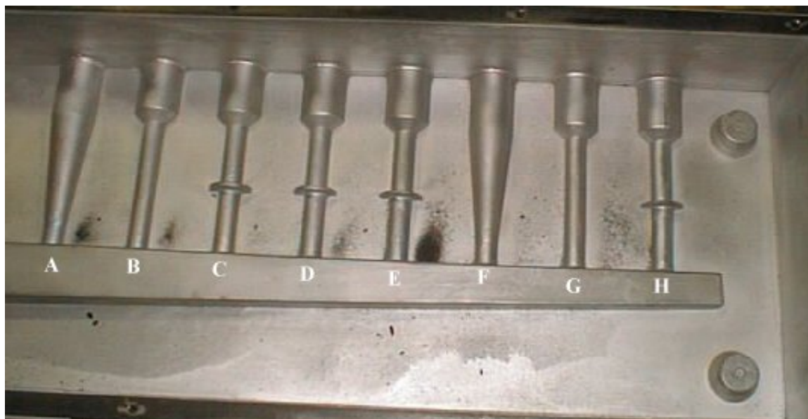
Figure 2.1 - Photograph of Pattern with Individually Labeled Blanks
