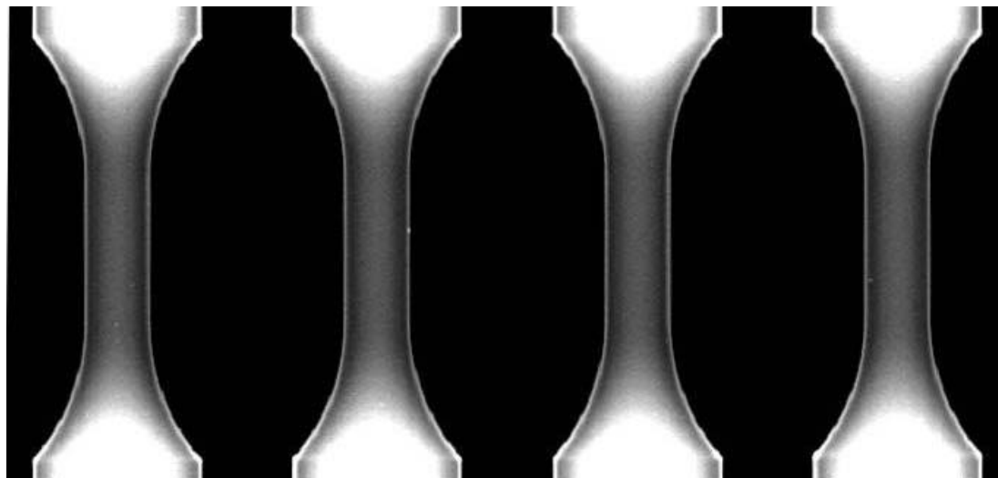
Figure 2.5 - Representative Radiographs of Truncated Cone Specimens
