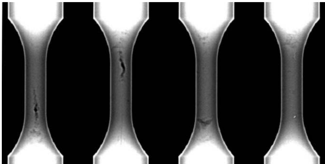
Figure 2.7 - Representative Radiographs of Cylinder with 5 mm Disc Specimens
